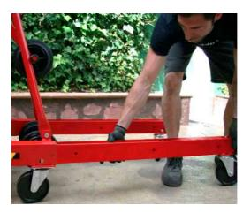
3.- Insert the magnetic locking pins and adjust the levelling jacks until the legs are firm and free of wobbling.
