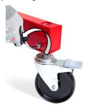
4.3.- Adjust the levelling jacks until the legs are firm and free of wobbling, levelling the lifter from the front axis with the help of the spirit level.
