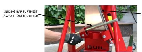
SLIDING BAR CLOSEST TO THE LIFTER 5.2.- Press the blocking lever that protrudes from the bottom of the adjusting box and at the same time unfold the outriggers down to the ground.
