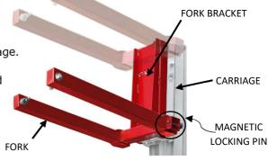
5.- Install the forks in the working position.
