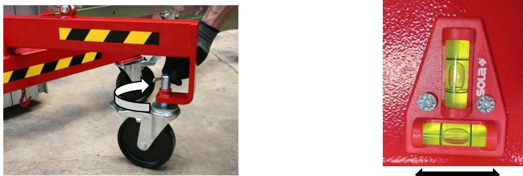
6.- Remove the profile blocking hook by twisting the central part to lengthen it and unhook it from the eye nut.
