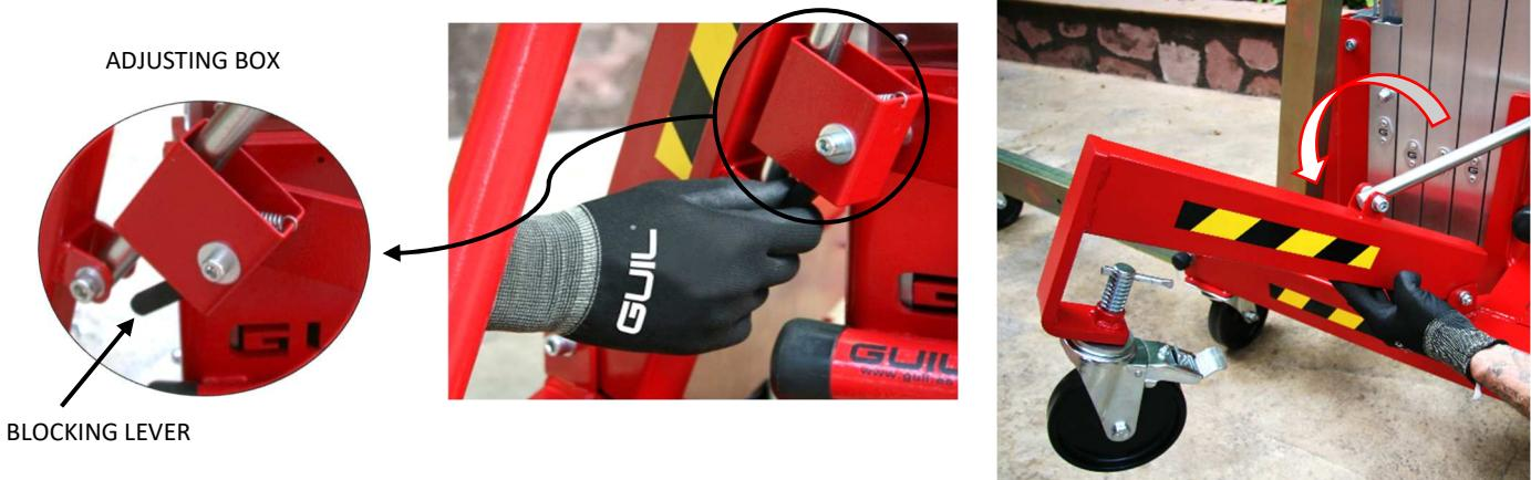
5.3.- Adjust the levelling jacks until the legs are firm and free of wobbling, levelling the lifter from the sideways axis with the help of the spirit level.
