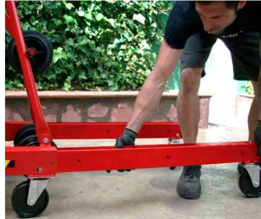
3.- Insert the magnetic locking pins and adjust the levelling jacks until the legs are firm and free of wobbling.
