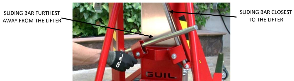
5.2.- Press the blocking lever that protrudes from the bottom of the adjusting box and at the same time unfold the outriggers down to the ground.
