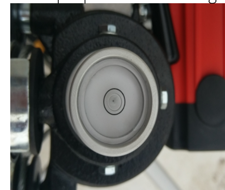
Mast level indicator
