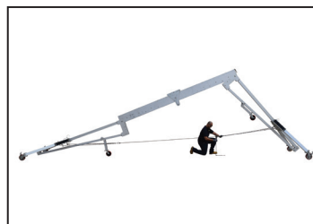
Ratchet 1st A-Frame bolt to beam.
